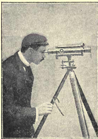
FIG. 129.—How NOT to use a level.
